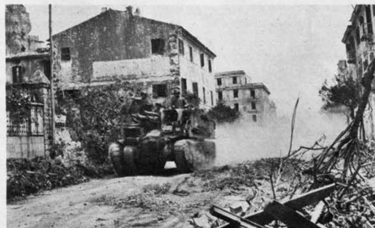
The suspension system of this U. S. M-7 rumbling through dusty Terracina on the road to Rome is same as that of the M-4 (above).
